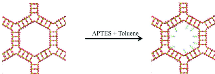
Figure 5. Schematic diagram illustrating the functionalization of MCM-41 by A) co-condensation and B) post synthesis grafting.
